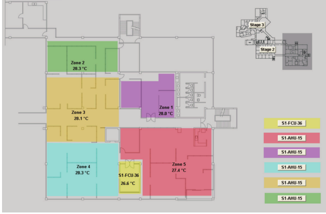
Figure 1: Schematic of floor layout and the thermal zones. Climate control to this section is provided by one AHU.
