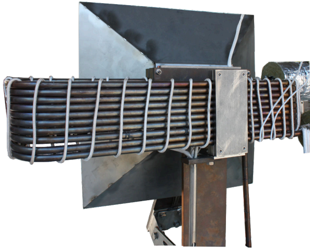
Figure A.18: Rear view of receiver with trace heating elements and without insulation. Frank Fellmoser 2018
