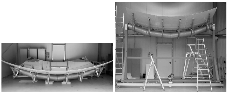
Figure 4.5: Parabolic mirror prior to (left image) and after mounting (right image) on support frame.
