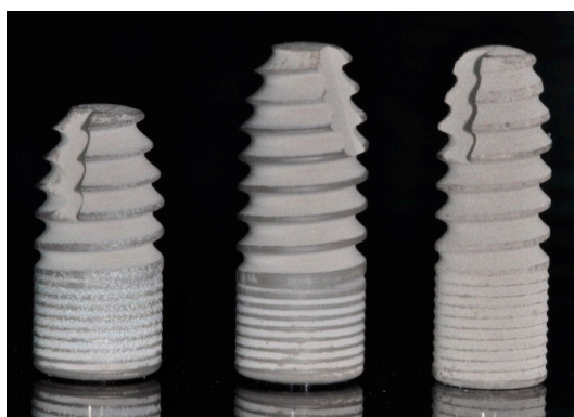
Figure 1. Implant dimensions used in this study: (left) implant dimension 4.8 \times 10 mm; (middle) implant dimension 4.8 \times 12.5 mm; (right) implant dimension 4.1 \times 12.5 mm.
