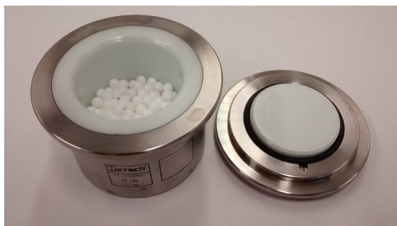
Figure 1.5: Typical zirconia grinding vial by Retsch , with 200 zirconia milling balls. The vial has a volume of 45 mL, the balls have a diameter of 5 mm and a weight of approximately 80 g.
