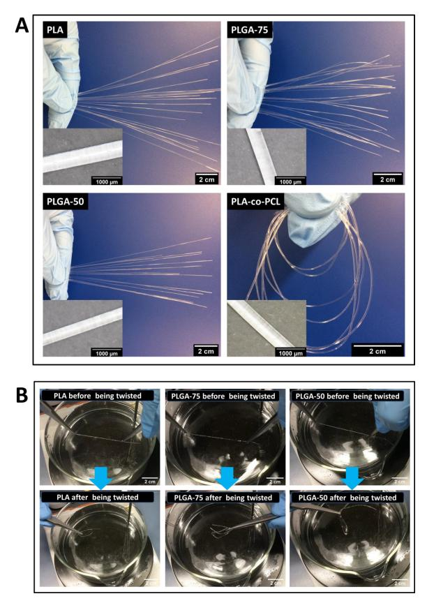
**Figure 3.** (A)Images of printed optical fibers from PLA and its copolymers. Insets show magnified images of the fibers demonstrating shape fidelity and
