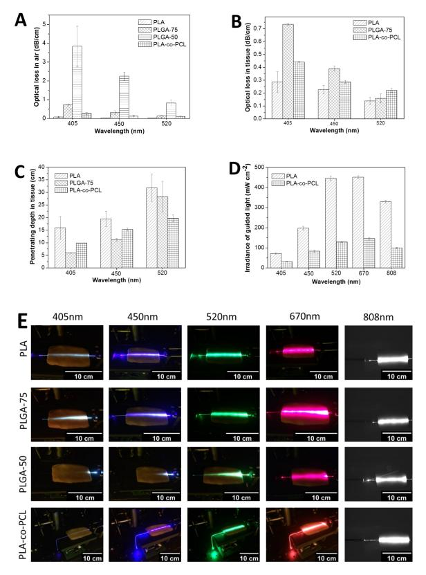
**Figure 4.** (A) Optical loss of printed waveguides in air; (B) Optical loss of printed waveguides in tissue; (C) Penetration depth of guided light in tissue; (D) The irradiance of light at the distal end of fiber (10 cm) that sandwiched by porcine
