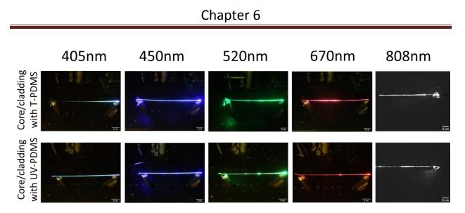
Figure A8. Images of light guided by printed waveguides in air, scale bar: 2 cm.
