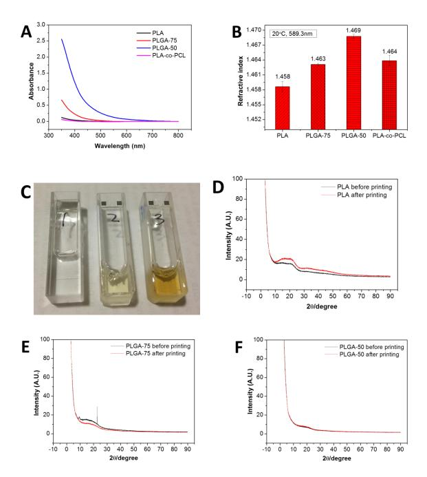
**Figure 1.** (A) Absorbance spectra of PLA, PLGA-75, PLGA-50 and PLA-co-PCL (B) Refractive index of PLA, PLGA-75, PLGA-50 and PLA-co-PCL measured at 589.3 nm and 20°C. (C) The color of melted PLA (1), PLGA-75 (2) and PLGA-50 (3). (D-F) XRD patterns of the polymers as powders and printed fibers.
