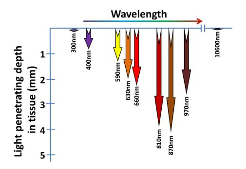
**Figure 7**. Light penetrating depth in skin tissue with different wavelengths. The image is adapted from ref<sup>[1b]</sup>.
