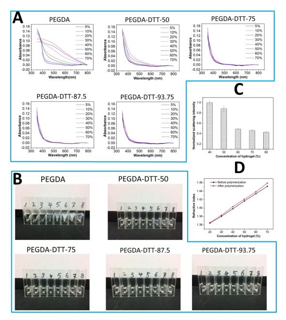
**Figure A2.** (A) Absorbance of PEGDA-DTT hydrogels at different concentrations; (B) Images of PEGDA-DTT hydrogels in (A). Numbers 1 to 8 stand for the polymer concentration in the hydrogels: 1-70wt%, 2-60wt%, 3-50wt%, 4-40wt%, 5-30wt%, 6-20wt%, 7-10wt%, 8-5wt%; (C) The relative scattering of PEGDA-DTT-87.5 hydrogels at different concentration; (D) The refractive index of PEGDA-DTT-93.75 hydrogels at different concentrations before and after polymerization.
