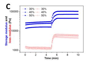
**Figure A7.** (A) <sup>1</sup>H NMR of Pluronic F127. (B) <sup>1</sup>H NMR of Pluronic-DA. (C) The storage and loss modulus of Pluronic-DA solutions at different polymer concentrations before (0-5min) and after (5-10min) photoinitiated covalent crosslinking.
