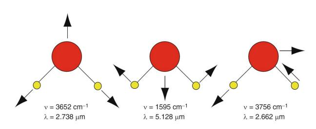
**Figure 3**. Different vibration modes of a water molecule with different absorption bands. Reprinted after permission from ref<sup>[8]</sup>. Copyright © 2011, Springer-Verlag Berlin Heidelberg.
