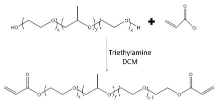
**Scheme A1.** The reaction between Pluronic F127 and acryloyl chloride to form Pluronic-DA.
