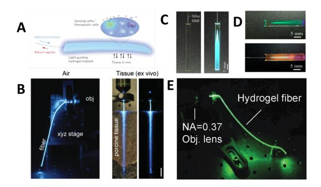
**Figure 11.** (A) Scheme of a hydrogel based waveguide with engineered cells for in vivo sensing and therapy encapsulated inside. Environmental stimuli can trigger cells in the waveguide to generate luminescence (achieve sensing) and external
