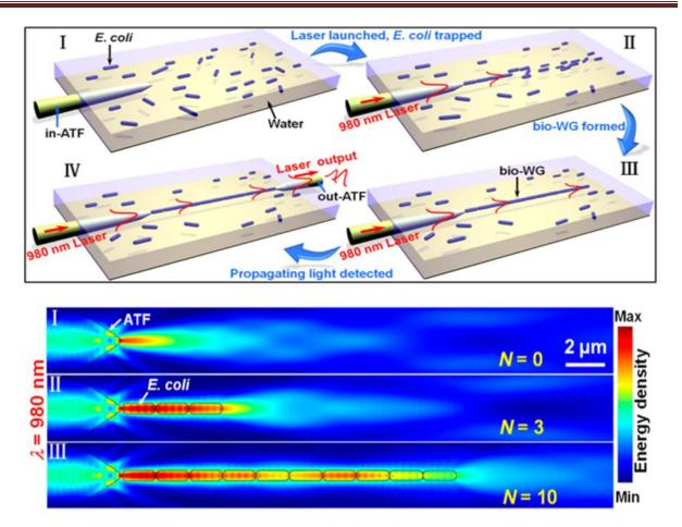
**Figure 9.** Up: Scheme of trapping E.coli and its light guiding. I, placing the in-ATF in a E. coli suspension; II, launching 980 nm laser into the in-ATF, E. coli starts to be trapped; III, The trapped and connected E.coli forming a bio-WG; IV, guided light is received by an out-ATF. Below: Energy density distribution in the ATF with different number (0, 3 and 10) of trapped E. coli. Reprinted after permission from ref<sup>[55]</sup>. Copyright © 2013, American Chemical Society.
