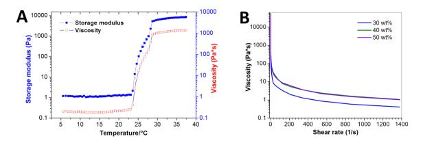
**Figure 1.** (A) The storage modulus and viscosity of 20 wt/v% Pluronic-DA in a temperature sweep rheology experiment (5 – 37 °C). (B) The viscosity of different concentration of Pluronic-DA at increasing shear rate.
