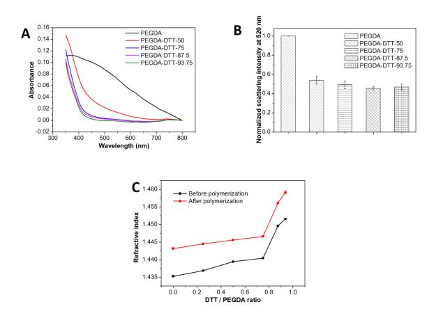
**Figure 2.** Optical properties of PEGDA-DTT hydrogels. (A) UV-Vis spectrum of 10 wt% PEGDA-DTT hydrogels. (B) The relative scattering of 70 wt% PEGDA-DTT hydrogels with different DTT/PEGDA ratio; (C) The refractive index of 70 wt% PEGDA-DTT based hydrogels before and after polymerization.
