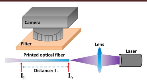
**Scheme 2**. Home-made setup to characterize the light guiding properties of printed optical waveguides.
