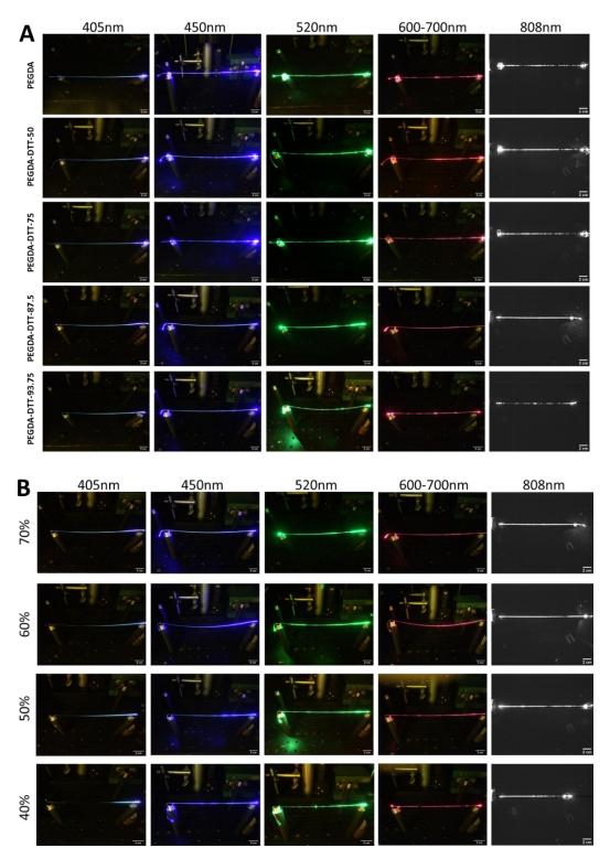
**Figure A3.** (A) Images of light guided through printed PEGDA-DTT waveguides in air; (B) Images of light guided through printed PEGDA-DTT-87.5 waveguides at different concentration in air.
