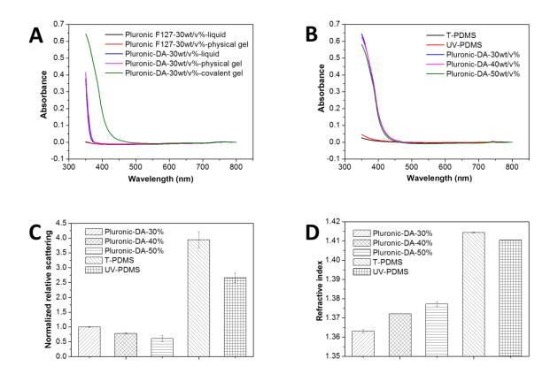
**Figure 2.** (A) Absorbance spectra of Pluronic F127 and Pluronic-DA solutions and their physical and covalent hydrogels. (B) Absorbance spectra of cured PDMS and
