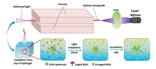
**Scheme 3.** Proof-of-principle scenarios for the application of PEGDA-DTT optical waveguides. Top part: Setup used to deliver light to a targeted destination by waveguides through tissue. 3D culture of a fibroblast spheroid within a polymeric matrix modified with photoactivatable cell adhesive ligands. After exposure fibroblasts sense the light-activated cell adhesive ligand and migrate out of the spheroid.
