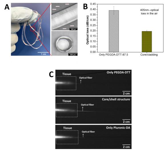
**Figure 7.** (A) Images of printed core/cladding fibers (80 wt% of PEGDA-DTT-87.5 for core, 50 wt/v% of Pluronic-DA for cladding). Left: printed core/cladding fibers, right: magnified images of core/cladding fiber and the cross-section of the fiber.
