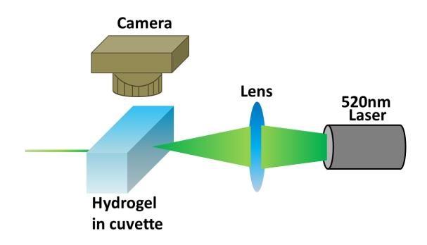
**Scheme 1**. Home-made setup to characterize the relative scattering of PEGDA-DTT hydrogels.
