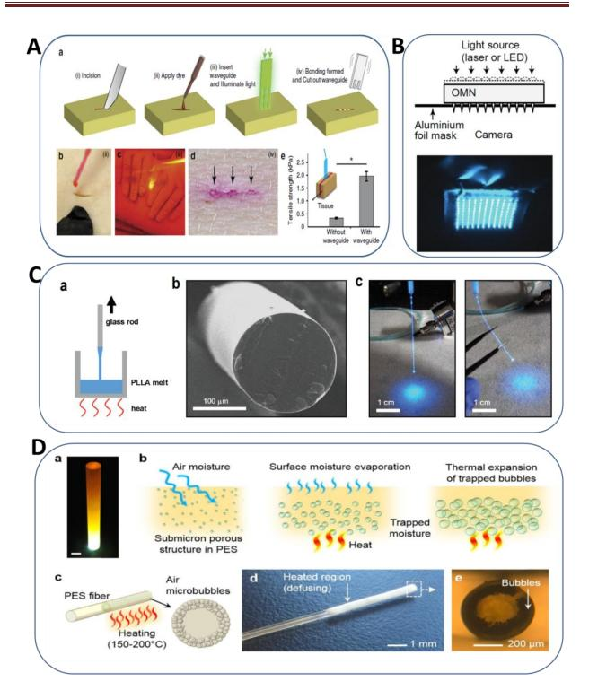
**Figure 10.** (A) a: Scheme of applying waveguides to deliver light into deep tissue to activate tissue glue. (i) Cutting skin incision; (ii) Applying Rose Bengal dye to the wound and removing extra solution; (iii) A delivering light through a prepared optical waveguide into the wound; (iv) Trimming the waveguide part out of skin surface. b–d: Experimental operations of steps (ii), (iii) and (iv). (e) Shear tensile strength of PTB bonds with and without waveguide in porcine skin. The improved
