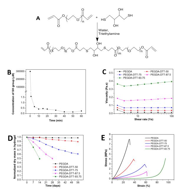
**Figure 1.** Chemical design and physical properties of PEGDA-DTT prepolymers and hydrogels (A) Synthesis of PEGDA-DTT polymer from PEGDA and DTT precursors. (B) Kinetics of the Michael addition reaction between acrylate groups of PEGDA and thiol groups of DTT as followed by a Fluorometric Thiol Assay Kit. (C) The viscosity of PEGDA-DTT solutions (50 wt%) measured at different shear rate at
