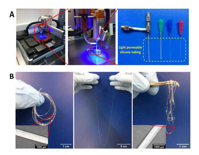
**Figure 3.** (A) Printing setup: left—printing stage of 3D-Bioscaffolder from GESIM, middle—printing head mounted with coaxial needle, right—printing needles extended with silicone tubes. (B) Images of printed 70 wt% PEGDA-DTT fibers with 510 μm silicone tube. Left PEGDA-DTT-50; middle PEGDA-DTT-87.5; right PEGDA-DTT-93.75 fiber. Scale bar of insets corresponds to 1000 μm.
