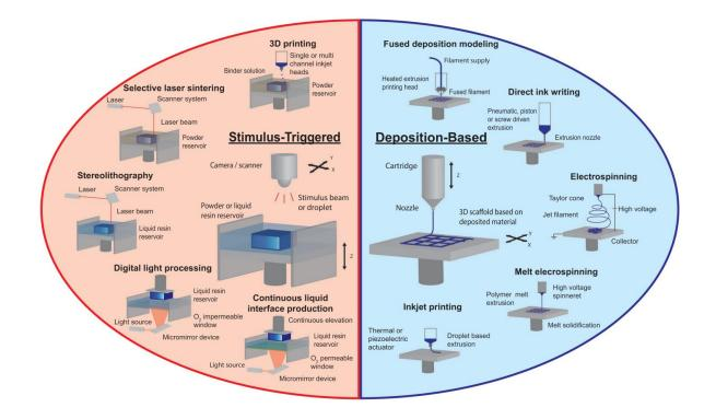
**Figure 15.** Classification of established 3D printing technologies available for the fabrication biomaterials. Left: Stimulus-triggered 3D printing technilogies; Right: Deposition-based 3D printing technologies. Reprinted after permission from ref<sup>[111]</sup>. Copyright © 2019 WILEY-VCH Verlag GmbH & Co. KGaA, Weinheim.
