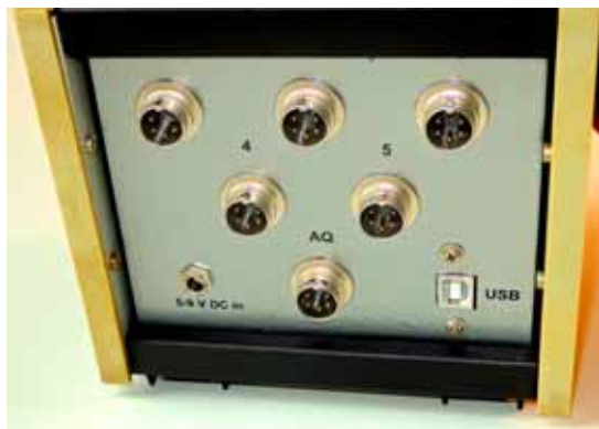
Picture 4. Rear panel of the sensor selector MPX-1.
