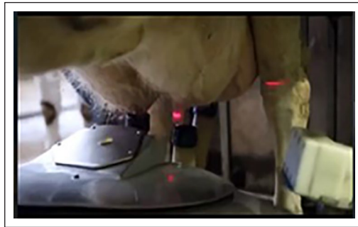
Image 10. ‘This is a state-of-the-art Merlin, an automatic laser guided milking robot’ (Greg Wallace, presenter).
