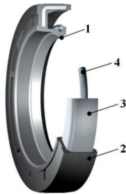
Figure 1. Radial Lip Seal Schematic [1] without dust lip to identify main components of this particular type of seal. 1. Sealing lip, 2. Outer static seal, 3. Supporting metal reinforcement, 4. garter spring.
