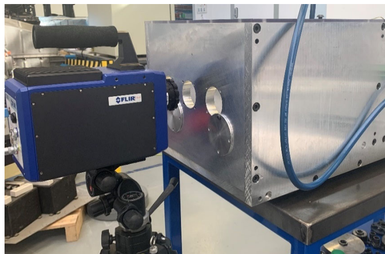
Figure 6. Set up of FLIR thermal imaging camera in front of the seal test bench.
