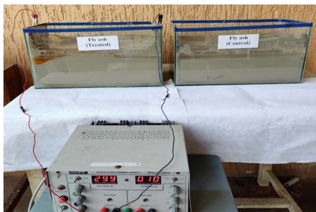
Fig 1. Experimental setup showing fly ash in electro dialytic cell, dual channel power supply.
