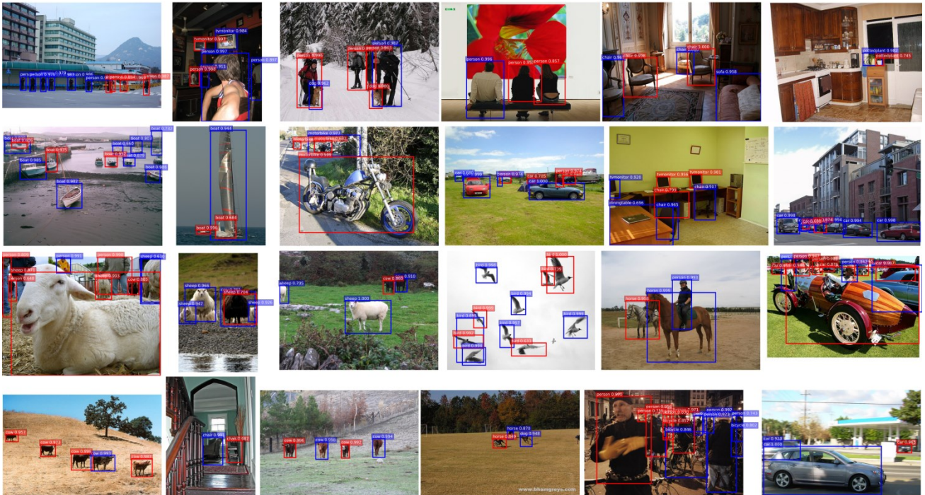
Fig. 4. Detection examples of K-Faster16 on the PASCAL VOC 2007 test set. A score threshold of 0.6 is used to draw the detection bounding boxes. The blue and red colors respectively show the detections launched by Faster and keypoint anchors.
