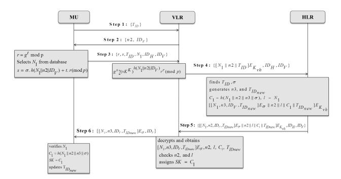
Fig. 1 The On-line Authentication Process of C.C. Lee et al.'s Protocol
