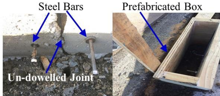
Figure 27. Steel bars used to attach LVDTs to PCC base and prefabricated wooden box enclosure to protect LVDTs from moisture damage.
