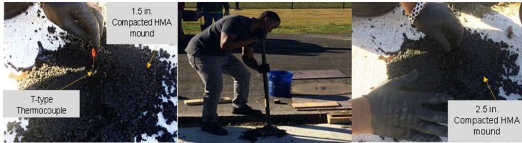
Figure 28. T-type thermocouple installation procedure.
