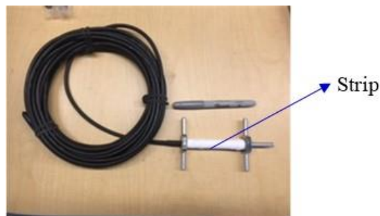
Figure 29. Picture of H-type, asphalt strain gauge installed in composite pavement sections.
