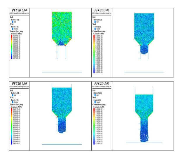
Figure 28. Contour plot for contact forces for nozzle size 200 μm and the needle length 0.25 mm.
