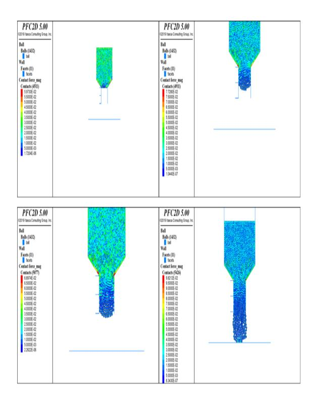
Figure A18. Contour plot for contact forces between for nozzle size  $400 \, \mu m$  and the needle length  $0.25 \, mm$ .
