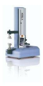
Figure 16. Compression Testing Machine
