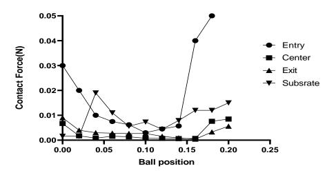
Figure 27. Contact forces vs. ball position graph at various locations of the model for nozzle size 200 µm and the needle length 0.25 mm.
