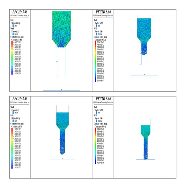
Figure A2. Contour plot for contact forces between for nozzle size 200  $\mu m$  and the needle length 0.25 mm.
