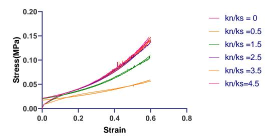
Figure 23. Stress-Strain curve at different Stiffness Ratio.
