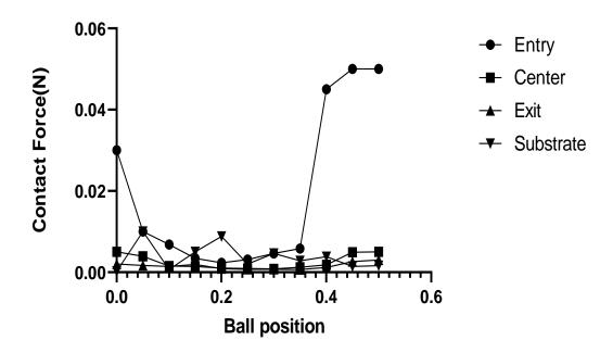
Figure A19. Contact forces vs ball position graph at various locations of the model for nozzle size  $500 \, \mu m$  and the needle length  $0.5 \, mm$ .
