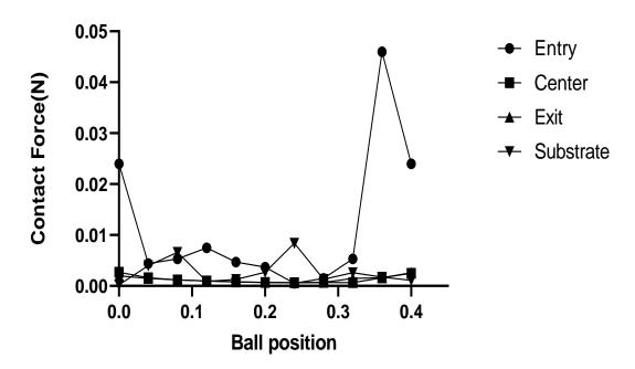
Figure A15. Contact forces vs ball position graph at various locations of the model for nozzle size  $400 \, \mu m$  and the needle length 1 mm.
