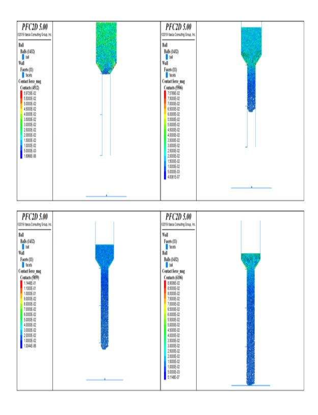
Figure A22. Contour plot for contact forces between for nozzle size  $500 \, \mu m$  and the needle length  $1.0 \, mm$
