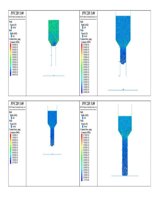
Figure A20. Contour plot for contact forces between for nozzle size  $500 \, \mu m$  and the needle length  $0.5 \, mm$ .
