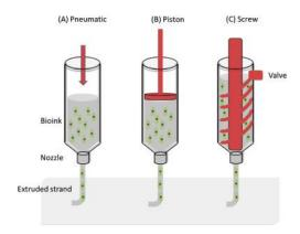
Figure 2. Extrusion based Bioprinting [19]
