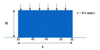
Figure 18. Uniaxial compressive test setup
