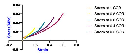
Figure 21. Stress-Strain curve with different Restitution Coefficients.
