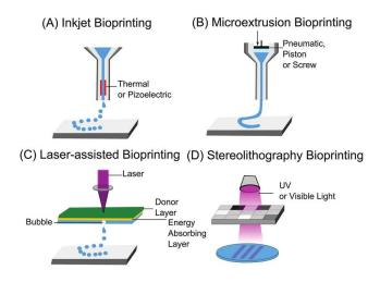
Figure 3. Various types of Bioprinting methods [33]
