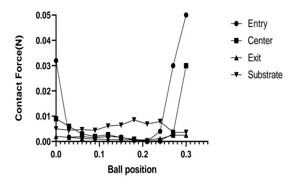
Figure A7. Contact forces vs ball position graph at various locations of the model for nozzle size 300 µm and the needle length 0.5 mm.
