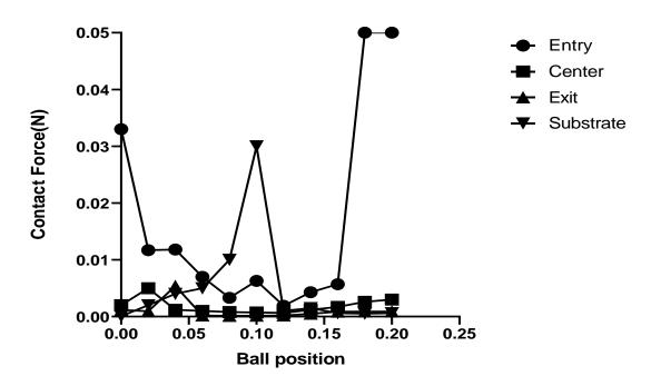
Figure A3. Contact forces vs ball position graph at various locations of the model for nozzle size 200  $\mu$ m and the needle length 1 mm.
