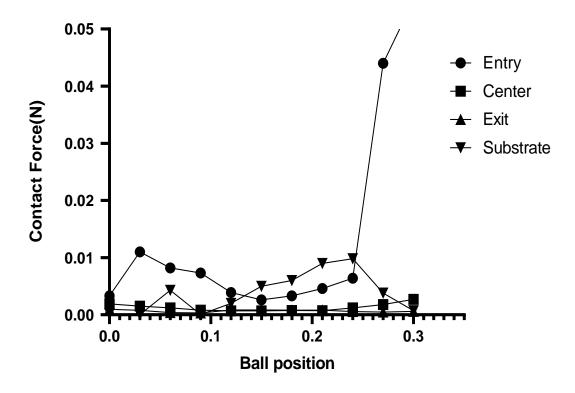
Figure A9. Contact forces vs ball position graph at various locations of the model for nozzle size 300 µm and the needle length 1 mm.
