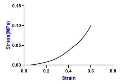
Figure 19. Stress-Strain under the confining pressure at 0.1 MPa
