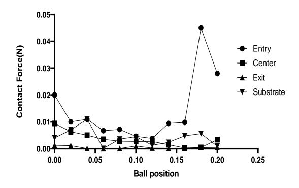
Figure A1. Contact forces vs ball position graph at various locations of the model for nozzle size 200  $\mu$ m and the needle length 0.5 mm.
