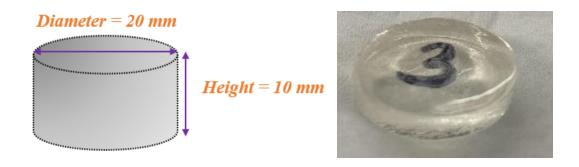
Figure 15. Specimen used for compression
