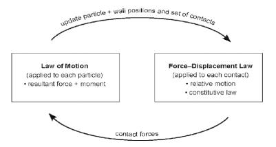
Figure 5. Calculation cycle in PFC<sup>2D</sup> [51]
