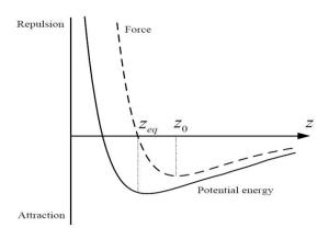
Figure 10. Potential energy and force between two molecules.
