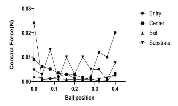
Figure A13. Contact forces vs ball position graph at various locations of the model for nozzle size  $400 \, \mu m$  and the needle length  $0.5 \, mm$ .
