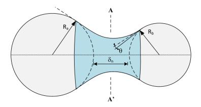
Figure 8. Capillary bridge model, A- A' shows the neck of the bridge.
