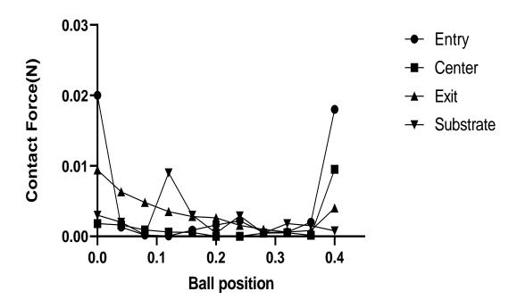
Figure A11. Contact forces vs ball position graph at various locations of the model for nozzle size  $400 \, \mu m$  and the needle length  $0.25 \, mm$ .
