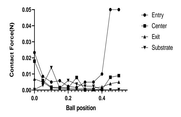
Figure A17. Contact forces vs ball position graph at various locations of the model for nozzle size  $500\,\mu m$  and the needle length  $0.25\,mm$ .
