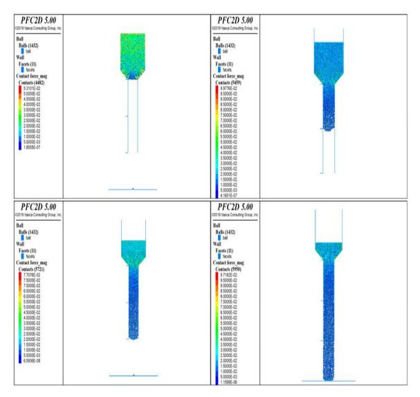
Figure A4. Contour plot for contact forces between for nozzle size 200  $\mu m$  and the needle length 1 mm.
