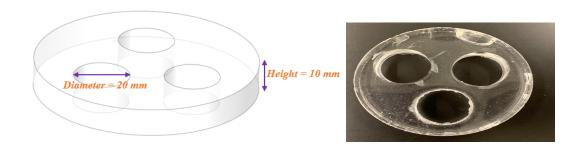
Figure 14. PDMS mold used for molding
