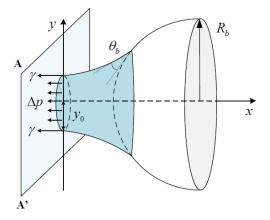
*Figure 9.* Capillary suction and surface tension in the liquid bridge at the cross-section A-A'.
