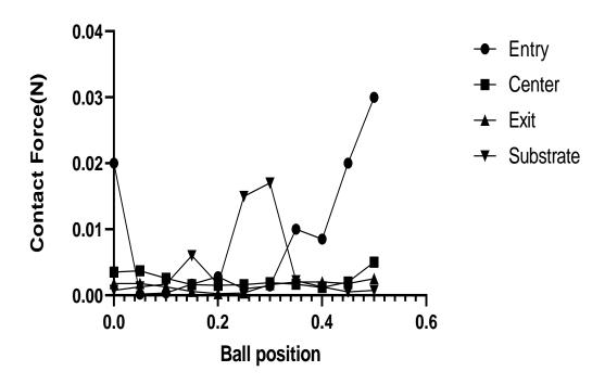
Figure A21. Contact forces vs ball position graph at various locations of the model for nozzle size  $500 \, \mu m$  and the needle length  $1.0 \, mm$ .
