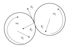
Figure 6. Decomposition of the contact force into the normal and tangential components.
