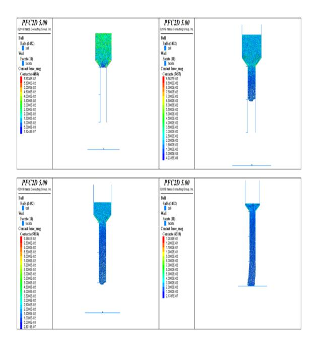
Figure A10. Contour plot for contact forces between for nozzle size 300  $\mu m$  and the needle length 1 mm.
