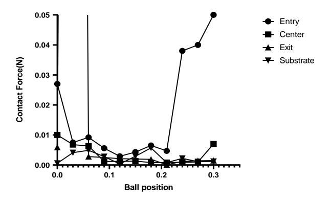
Figure A5. Contact forces vs ball position graph at various locations of the model for nozzle size  $300 \, \mu m$  and the needle length  $0.25 \, mm$ .
