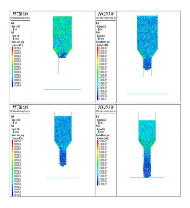
Figure A6. Contour plot for contact forces between for nozzle size 300  $\mu m$  and the needle length 0.25 mm.
