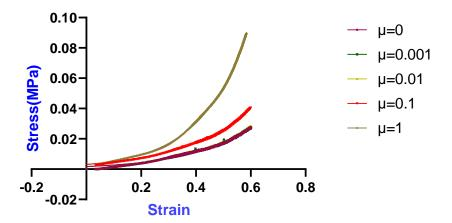
Figure 22. Stress-Strain curve with different Friction Coefficients.
