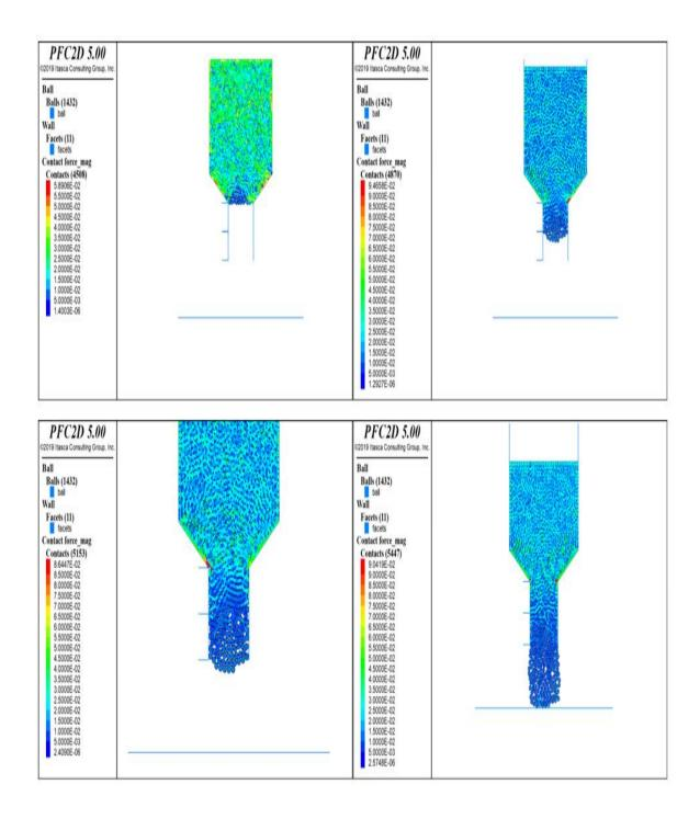
Figure A12. Contour plot for contact forces between for nozzle size  $400\,\mu m$  and the needle length  $0.25\,mm$ .
