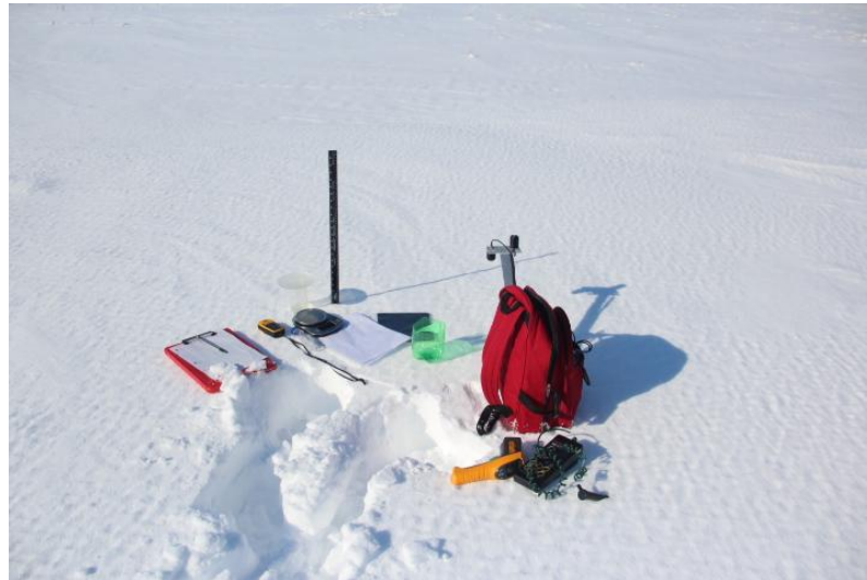
Figure 5. Instruments used for measuring physical properties of Snowpack: Common Ruler; Garmin Etrex GPS Unit; Weighing Scale; Fluke 561 IR Thermometer; Graduated Measuring Cylinder (1000ml); Container; Gridded Mesh Cards, Record Book; Pencil.
