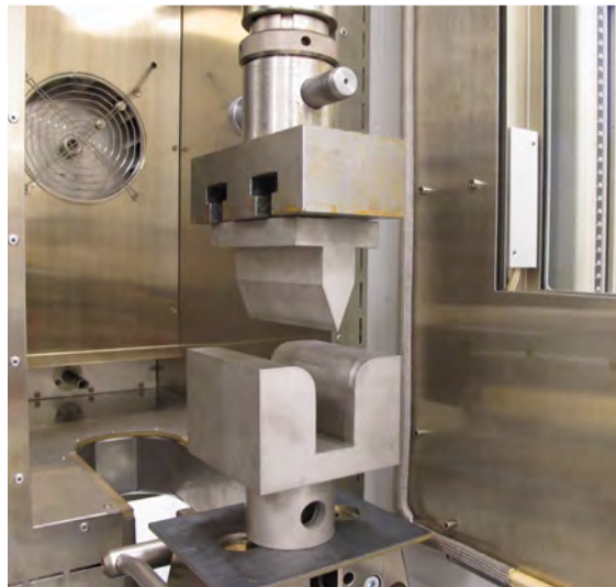
Figure 1. Pre-bending tooling assembly and the temperature chamber.
