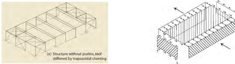
Figure 1. Example of a column and beam frame stiffened by sheeting and a diaphragm frame /14/ /17/
