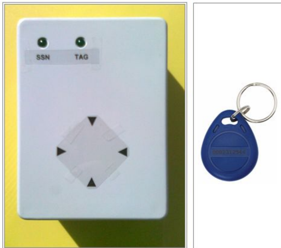
Figure 13. ID-Reader-Unit ( left ) and a compatible RFID tag ( right ) [12]
