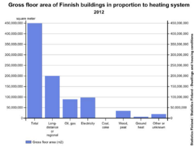
FIGURE 2-23. Gross floor area of Finnish buildings in relation to heating systems [23] (#cite-text-0-22)
