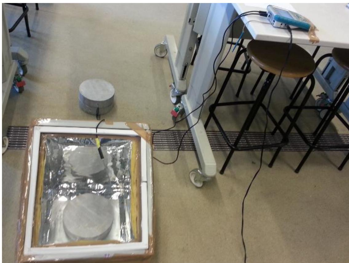
Figure 8. Experimental setup, Metropolia 1 box-type solar cooker insulation being tested
