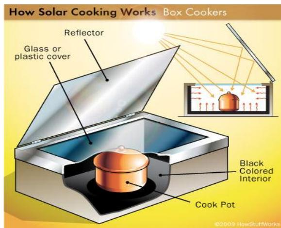
Figure 1. Box-type solar cooker (HowStuffWorks, 2009)
