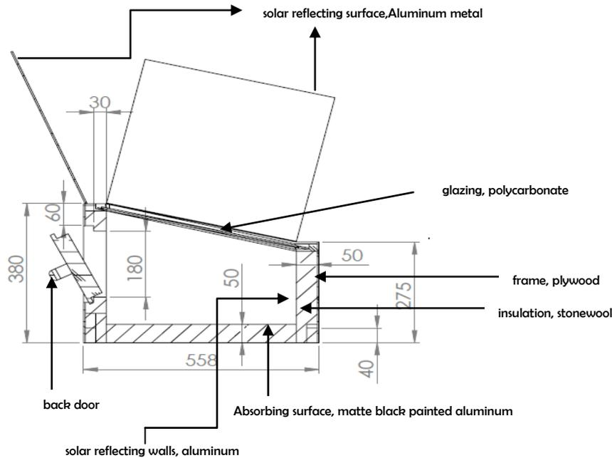
Figure 3. Sectional schematics of TEP ry's box-type solar cooker
