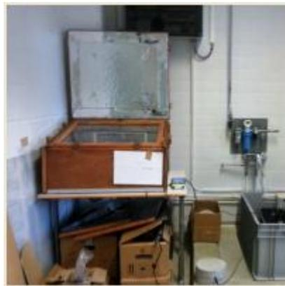
Figure 2. TEP ry's box-type solar cooker
