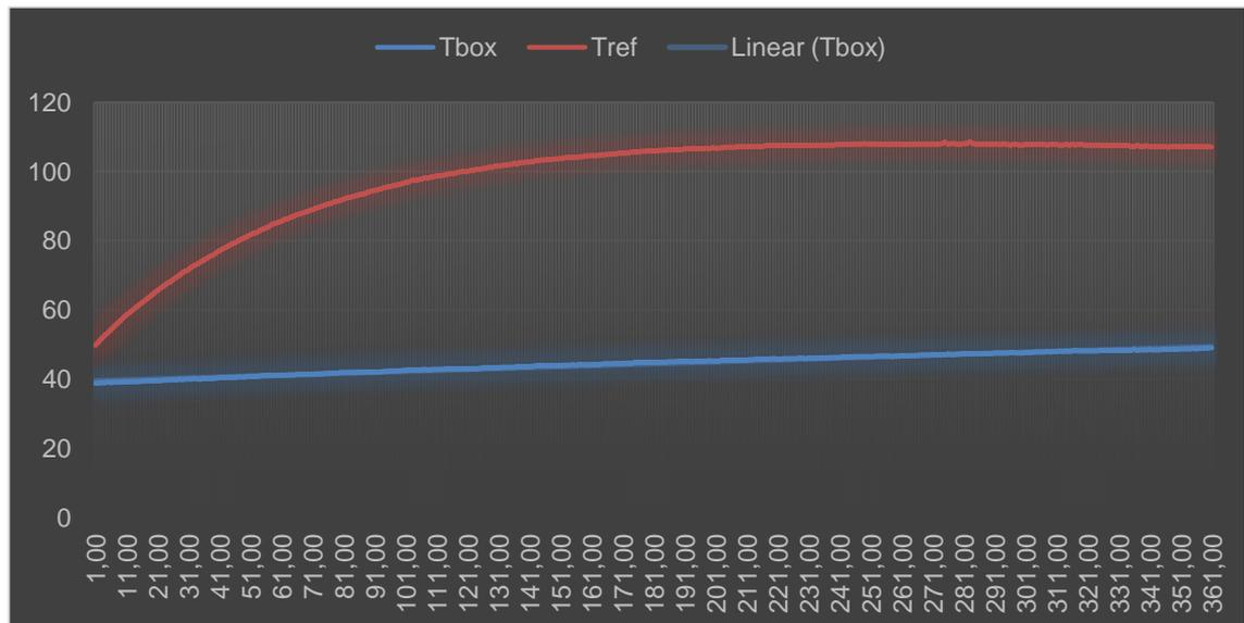
Figure 10. Time versus temperature plot for Metropolia 1 box-type solar cooker
