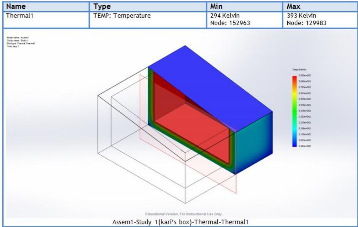
Figure 11. Thermal simulation results for TEP ry box-type solar cooker
