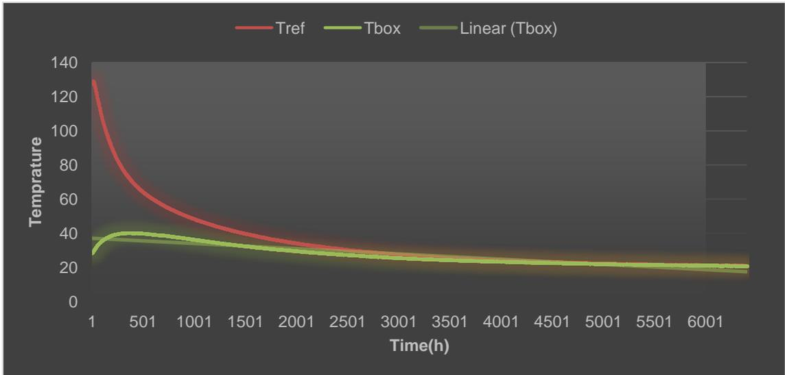
Figure 9: Time versus temperature plot for TEP's box-type solar cooker
