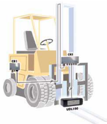
Figure 11: RFID reader's position on a forklift (ident, 2013)
