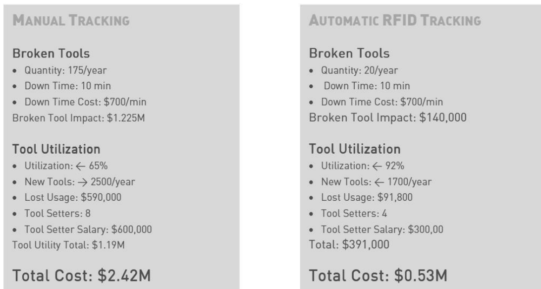
Figure 12: Manual tracking vs Automatic RFID Tracking (Xerafy, 2010)
