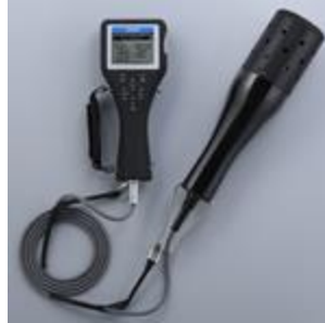
Figure 26. Multi-parameter Water Quality Meter, produced by Horiba. Source: Horiba corporate website (2014).
