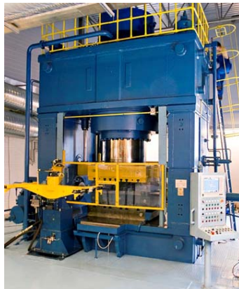
Fig. 14 - Hydroforming machine in Stainless Steel Studio. Ultimate force of the machine is 30 000 kN.
