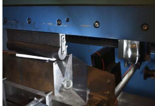
Fig. 10 - Pressing tool and measurement equipment. On the left there is the steel sheet being bent. On the right there are the light assembly and camera.
