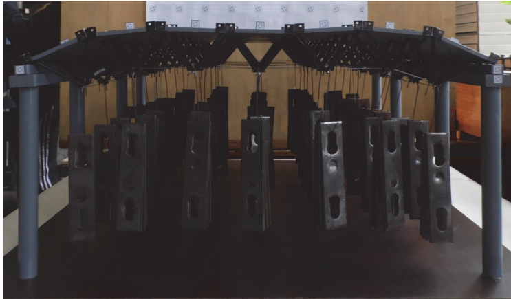
Figure 6. Deformed model diagram at full load
