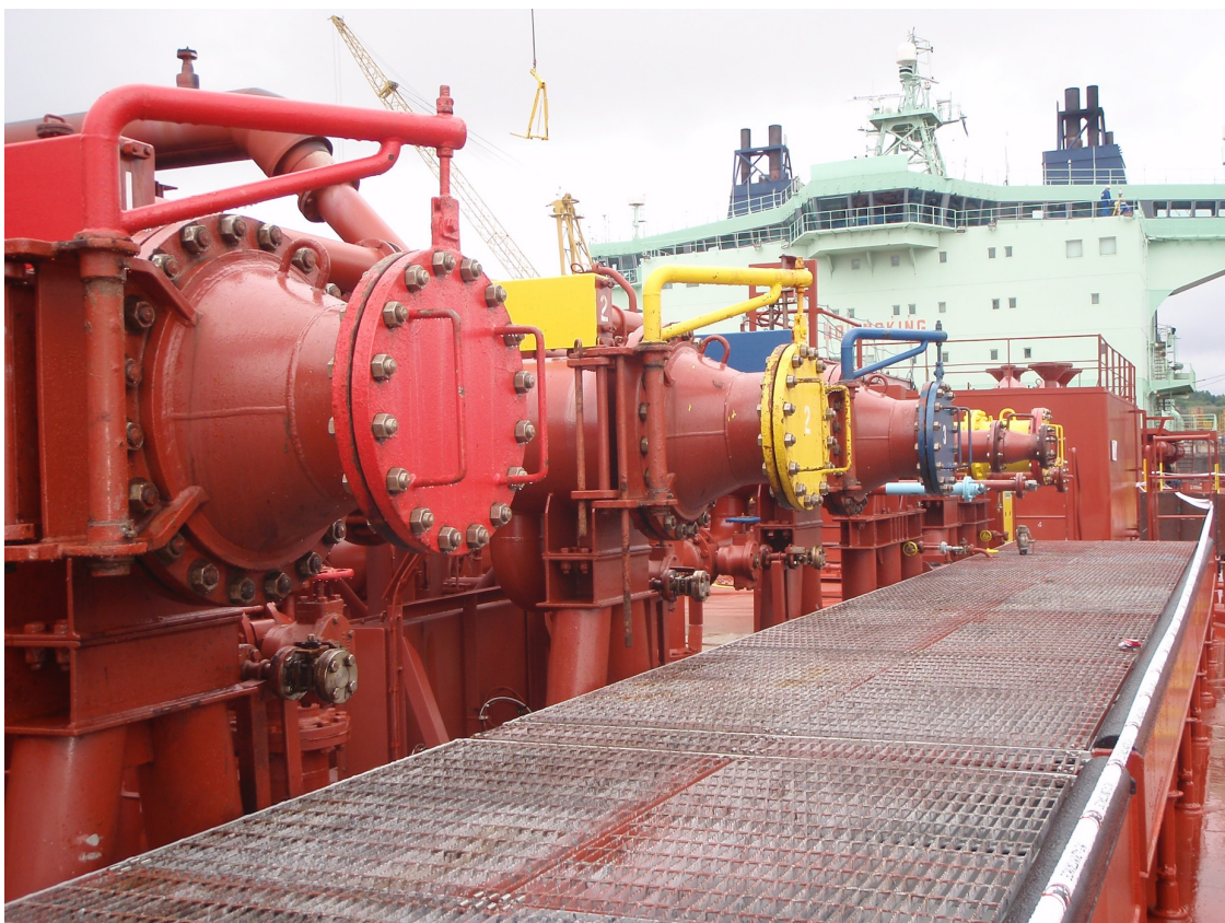
Picture 16. Manifolds of MT Tempera
