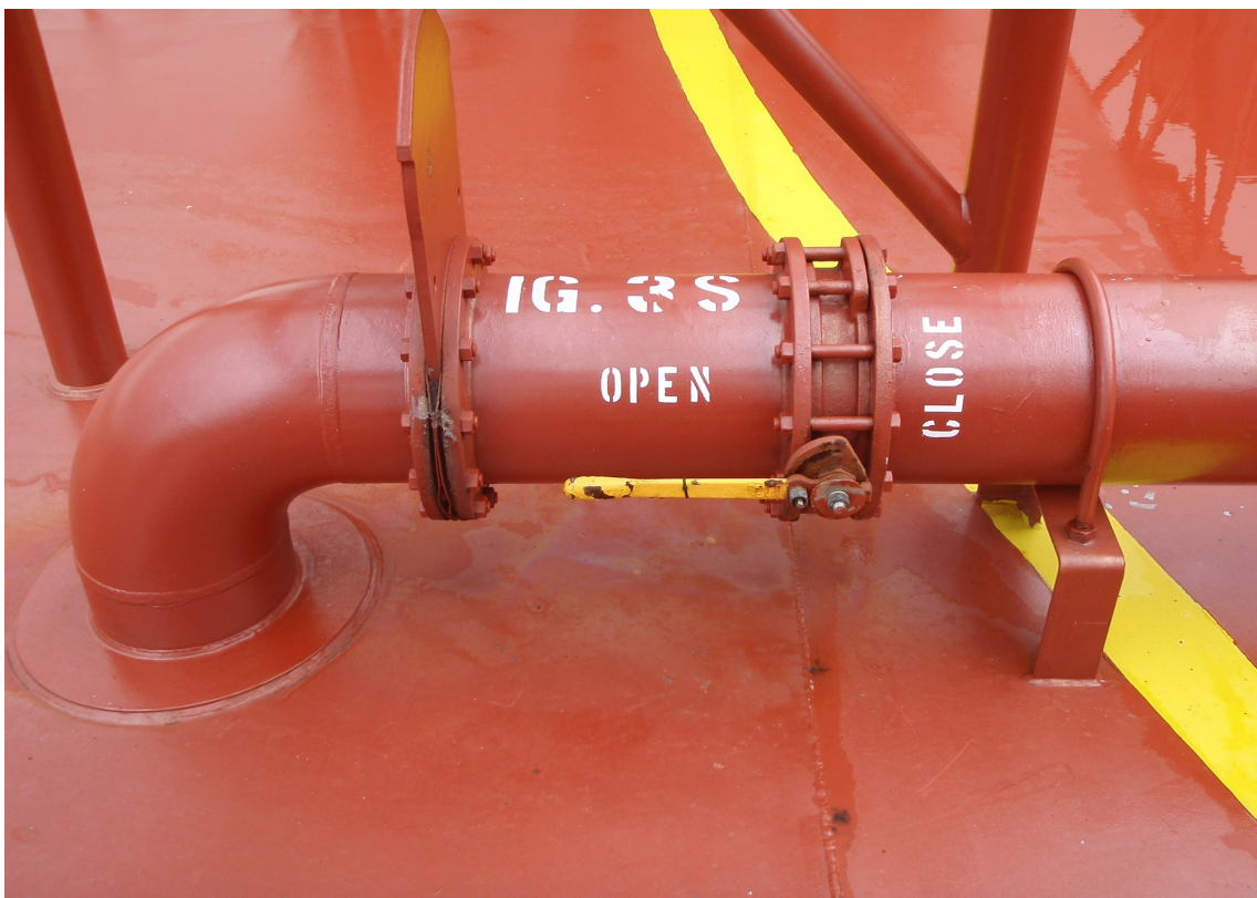
Picture 14. IG-line on board MT Tempera
