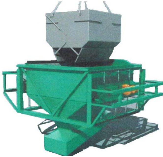
(Fig.12) Shaker (Source: Specifications for reprocessing of rubber waste "Constant 18M", 2006. 69.)
