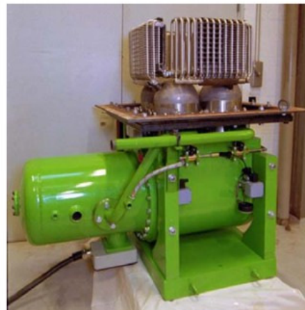
The newly developed 35 kW e Stirling engine for biomass combustion plants (Source: BIOS Bioenergy Systems, Austria & Henrik Carlsen, Denmark, 2003)
