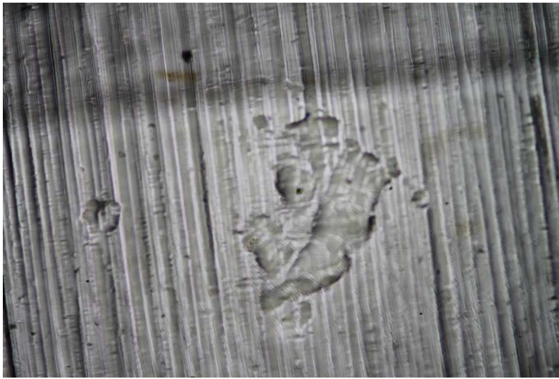
Figure 31 Spot that was found on all test pieces (Arcada 2013 Jonas Eklöf)
