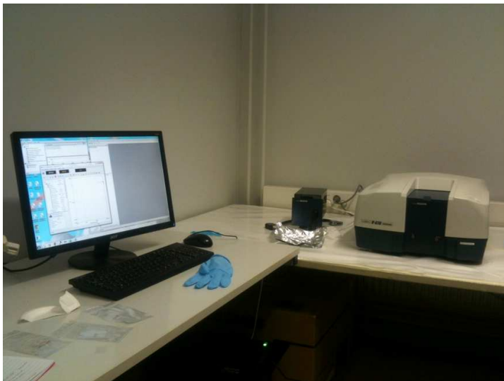
Figure 25 UV-NIR/VIS set up workstation. Software for calibrating results (left) and UV-NIR machine (right) (Arcada 2013 Jonas Eklöf)
