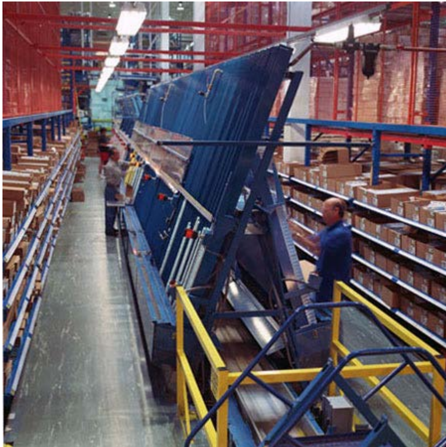
Figure 20. Automated split case order picking using an A-frame.
