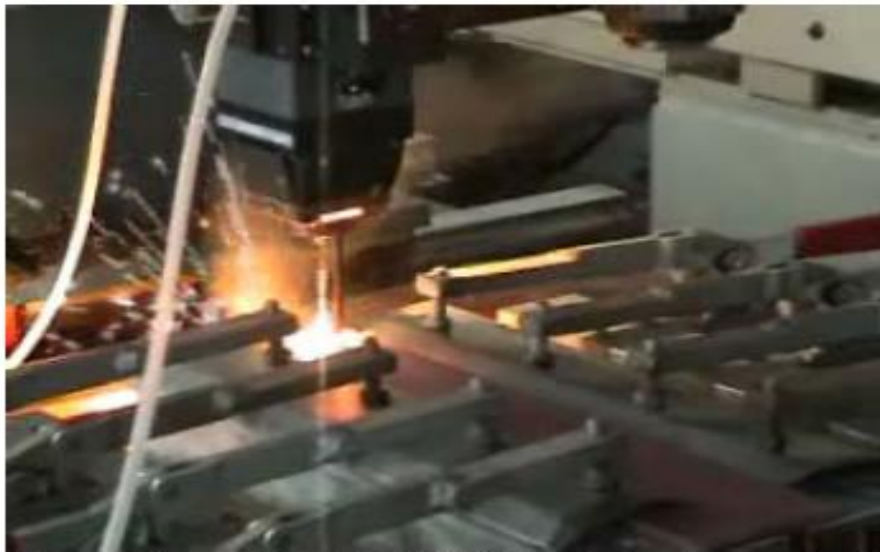
First welding tests with 10.4kW in steel using protective gas and cross jet
