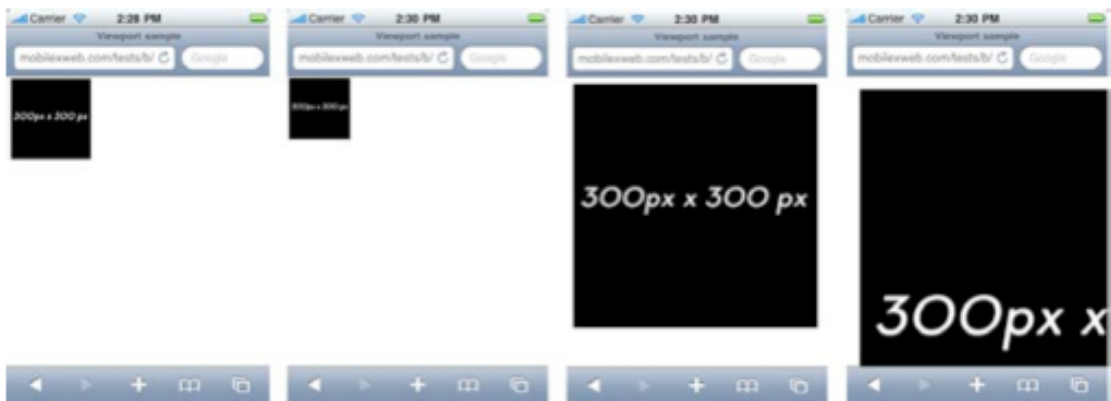
Figure 35. Viewing 300x300 pixel image in the default Safari viewport, in a 1500-pixel viewport, at a device-width set to the scale of 1.0 and at device-width set to scale 2.0. Copied from [4, 127].
