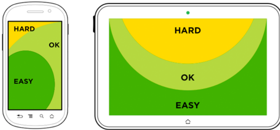
Figure 18. Interactions zones by difficulty on a smartphone and a tablet. Copied from [68].
