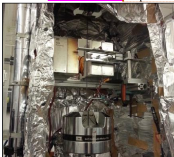
(a) MTS 810 Material Testing System (b) MTS 632.54F-11 Axial Extensometer Figure 1. Test equipment for tensile test of prestressing wire in and after fire
