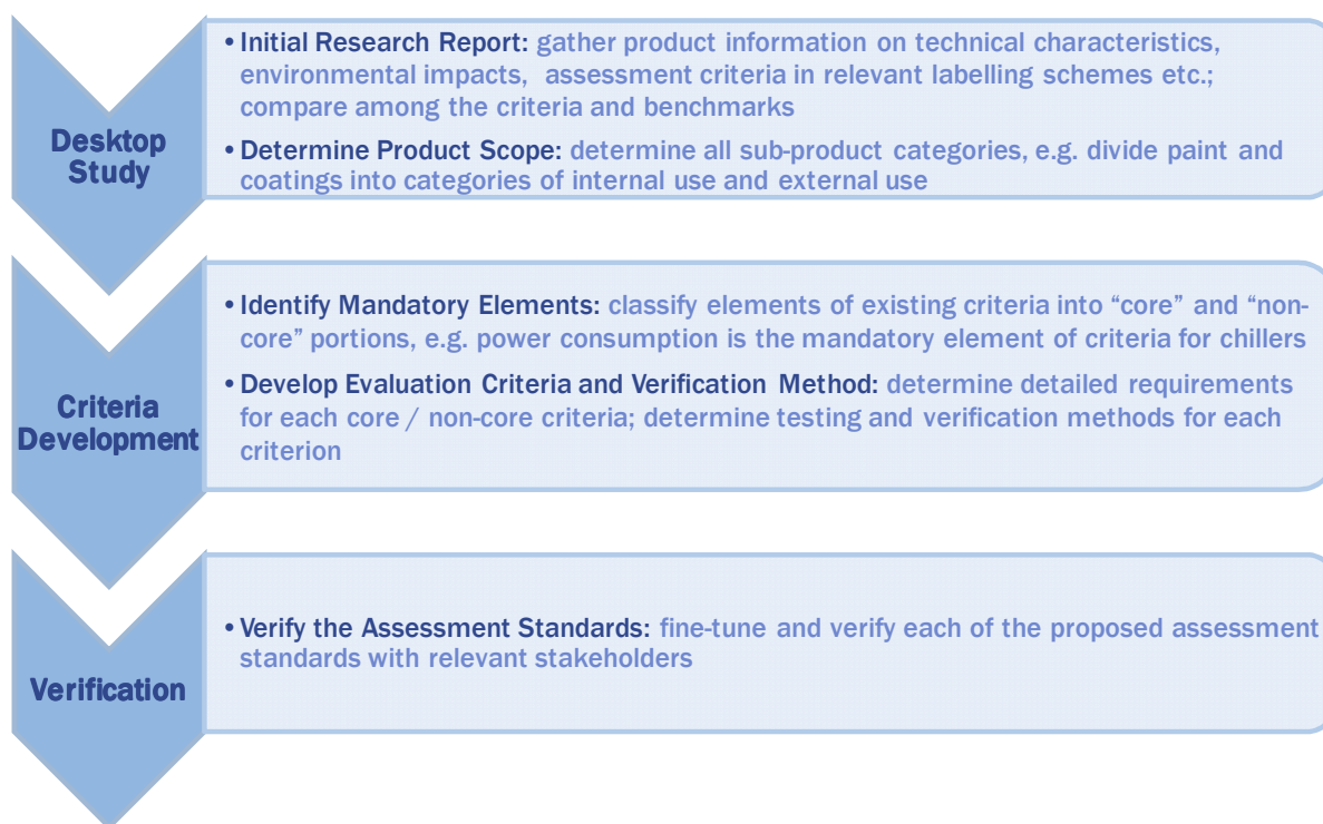
Figure 1: Stages involved in the development of the green building product labelling scheme
