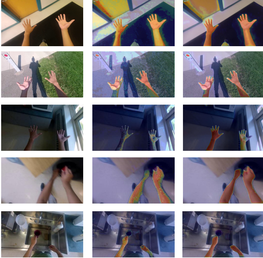
Fig. 6: Sample Images of EDSH data set: (left column) original images, (second column) results of Li's Method [15], and (last column) our results. From top to bottom: confusion with the door in EDSH1; shade on the hand in outdoor in EDSH2; poor light condition in EDSH2; motion blur in EDSH-Kitchen; confusion with sink in EDSH-Kitchen. Best view in color.
