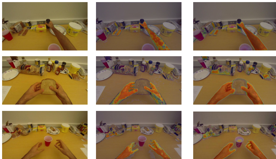
Fig. 5: Sample Images of GTEA dataset: (left column) original images, (second column) results of Li’s Method [15], and (last column) our results. From top to bottom: GTEA-Coffee, GTEA-Peanut and GTEA-Tea. Best view in color.
