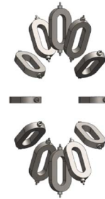
Fig. 5. Arrangement of cooling Dewars of the proposed machine.
