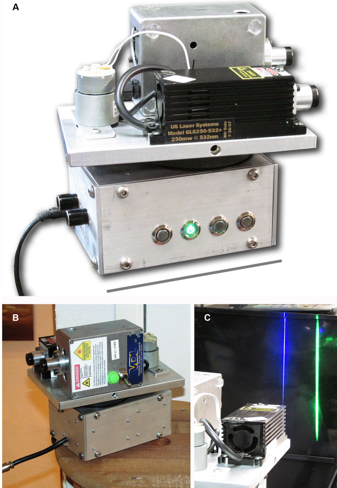
Fig 2. Laser scanning system. A, Custom-built laser scanning device. B, Blue and green laser modules are mounted onto the scanning plate. A variable speed DC motor scans the plate back and forth laterally and is adjustable for degrees covered. C, Removable line lenses convert the laser spot to a more diffuse vertical line. Scale bar in Fig 2A equals 15 cm.
