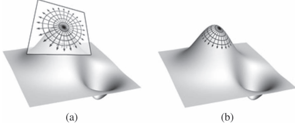
Fig. 2. The log/exp maps at point u introduces a mapping between a vector originating at u on \mathcal{T}_u and a geodesic beginning at u on \mathcal{M} . The circles on \mathcal{T}_u are mapped to the contours of the geodesic function on \mathcal{M} . (a) Coordinate system in \mathcal{T}_u (b) Coordinate system in \mathcal{M} .
