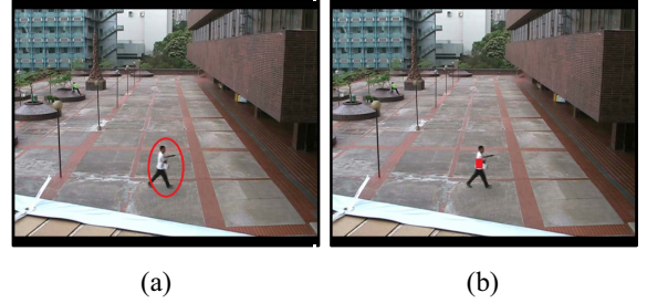
Fig. 5. Object initialization. (a) the object enclosed with a contour manually selected by user (b) auto selected blocks with local minimum/maximum motion vectors.
