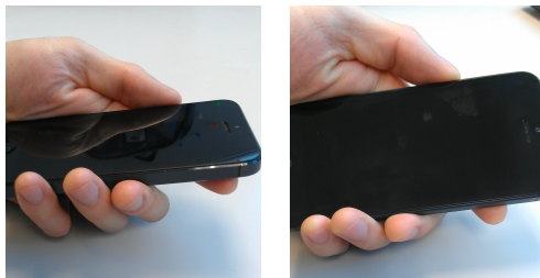
Figure 2. Gravity X gesture, which is used for switching to the next or previous page of notes determined by the chord-octave-scale combination at the next or previous square within the sequence.
