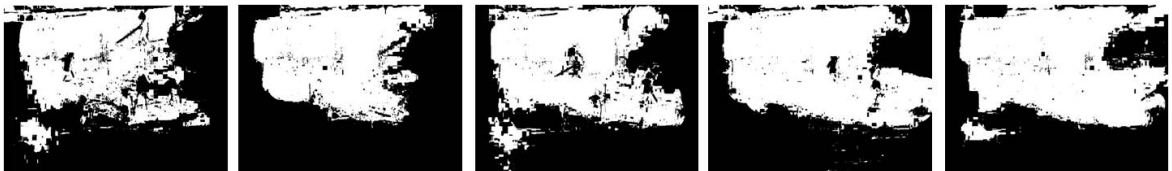
Figure 5 Extracted Concrete Region in the Testing Images
