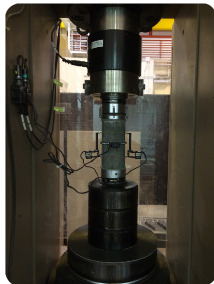
Static Elastic Modulus Test for Concrete Specimen
