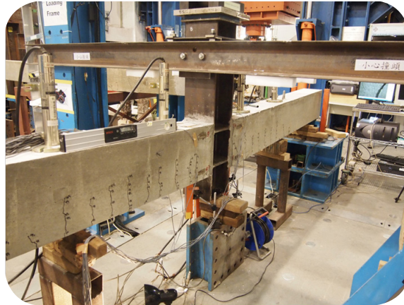
Figure 2 Testing of a Concrete Beam to Steel Column Connection
