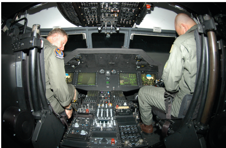
Figure 2. Simulator (high-fidelity simulation). Tactical Operation Flight Trainer is used for helicopter pilot training in U.S. Navy. (U.S. Navy photo by Mass Communication Specialist Seaman Michael C. Barton).
