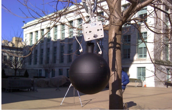
Figure A.1. The use of 150 mm (6-inch) black globe thermometer on Jan.15 2012 as a redundant experiment to evaluate the use of 40 mm grey globe thermometer. Photo taken Jan.15, 2012
