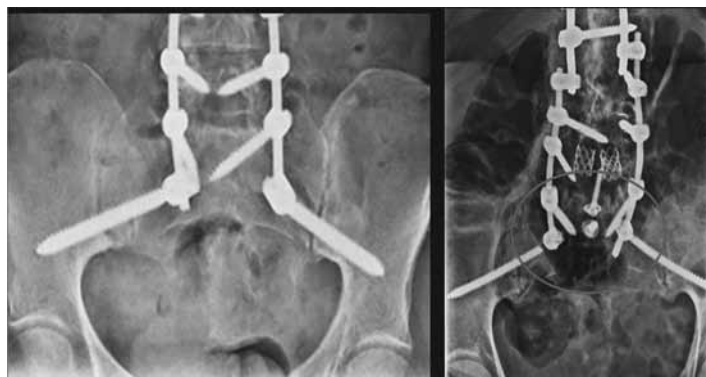
Radiograph showing fracture of the S2AI screws. All screws that fractured were 7 mm in diameter. No fracture was seen in 8mm or 9 mm screws (also shown).
