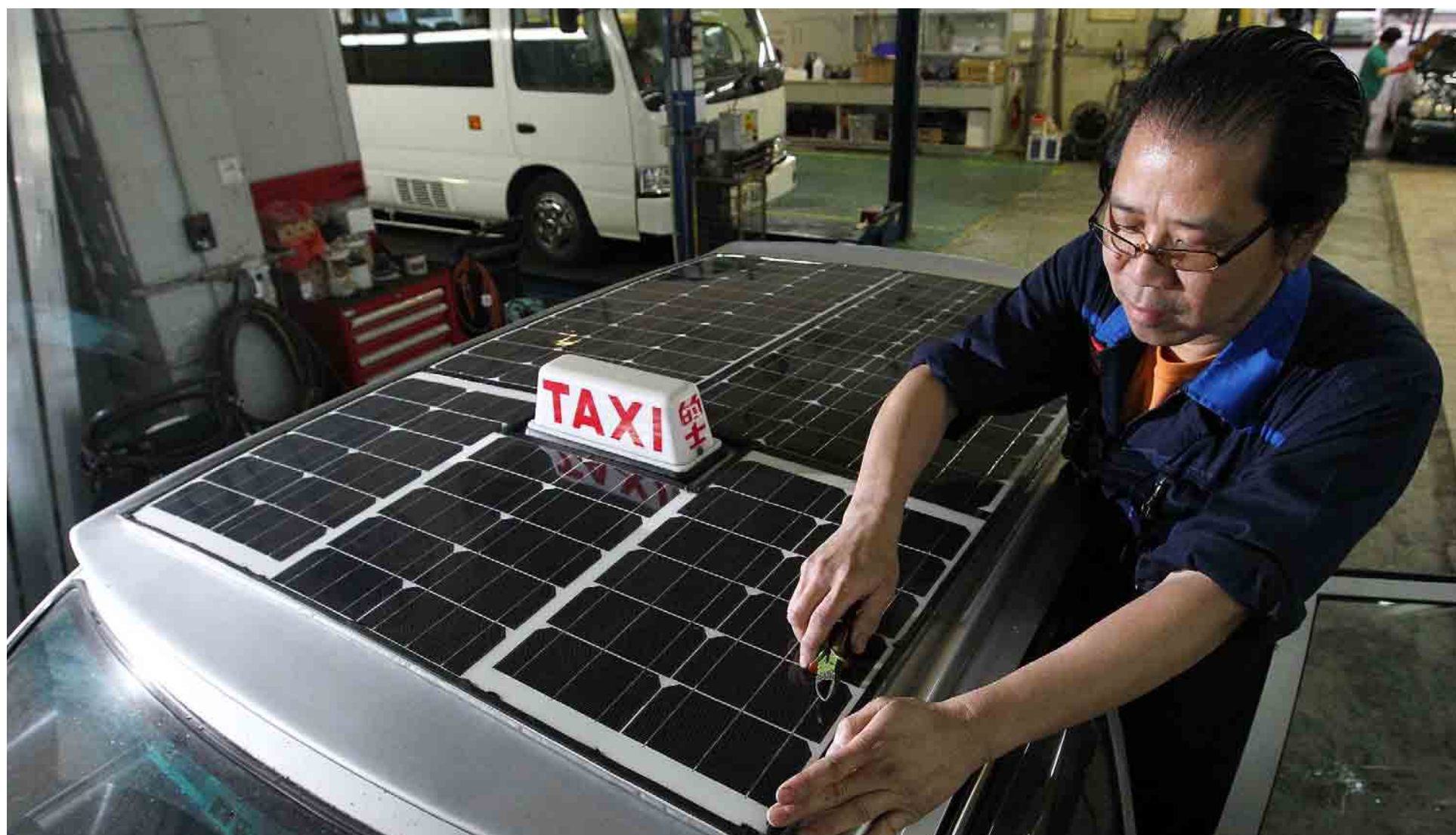
A taxi in Yuen Long is fitted with solar panels, integral to a new air-conditioning system made in Hong Kong. The panels convert solar power into electrical energy. Photo: May Tse
