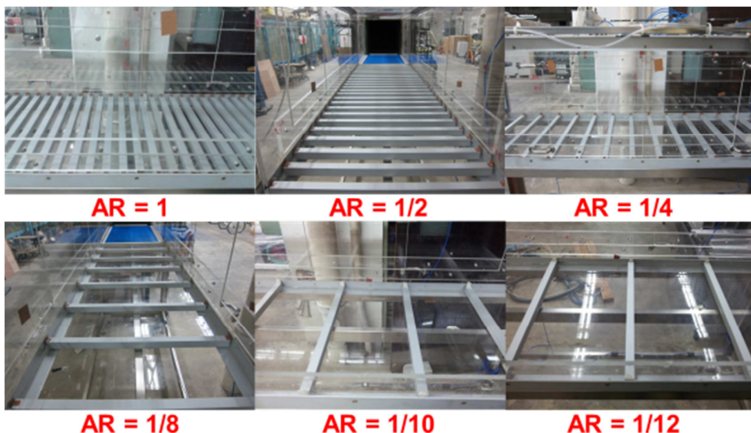
Figure 1: Different models of urban-type rough surface tested.
