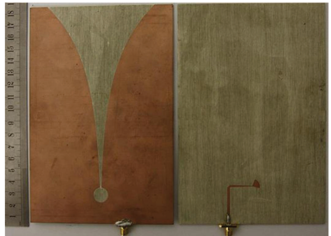
Figure 3c. The prototype of the reader's antenna.
