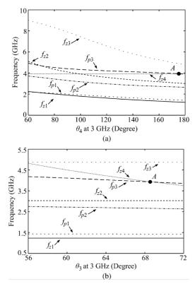
Fig. 3. Frequency locations of transmission poles and zeros versus electrical lengths of two open-circuited stubs. (a) When  $\theta_3 = 68.7^{\circ}$  at 3 GHz. (b) When  $\theta_4 = 176^{\circ}$  at 3 GHz. (Z<sub>1</sub> = 91.4  $\Omega$ , Z<sub>2</sub> = Z<sub>3</sub> = 115.1  $\Omega$ , and Z<sub>4</sub> = 135.4  $\Omega$ ).
