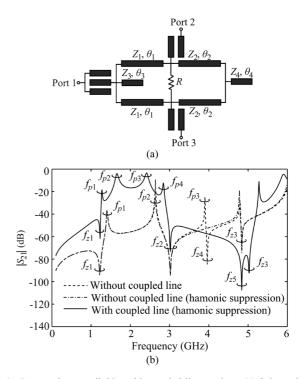
Fig. 4. Proposed power divider with coupled-line sections. (a) Schematic. (b) Frequency responses of S-magnitudes under the weak coupling.
