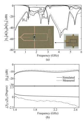
Fig. 6. Simulated and measured results. (a) S-Magnitudes. (b) Ports isolation and output phase difference with a resistor of 56  $\Omega$  in the measurement.
