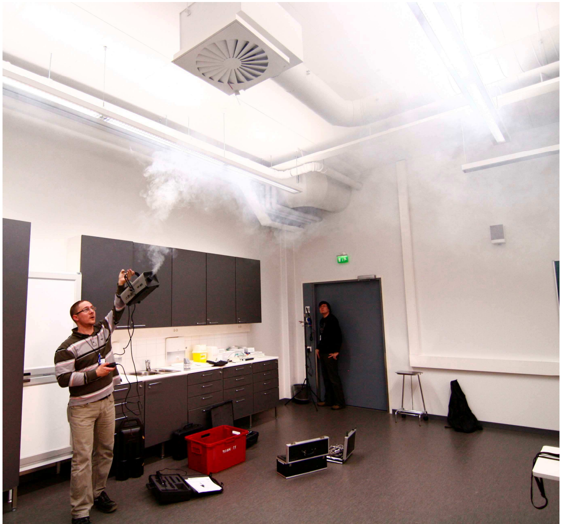
Figure 14. A air flow patterns determination with a smoke machine
