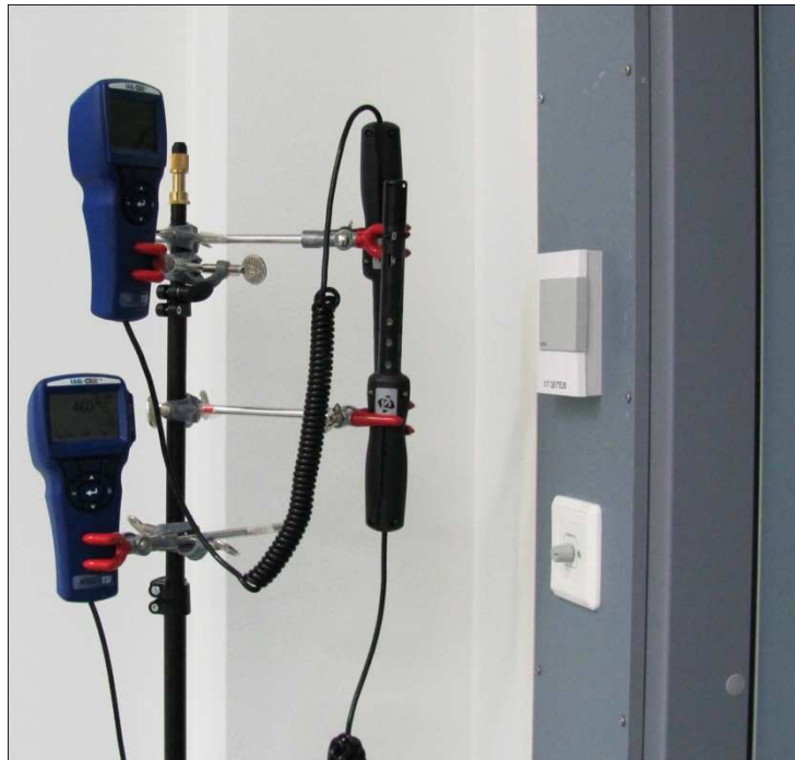
Figure 10. Picture of installation for comparing of three sensors results
