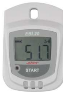
Figure 11. EBRO humidity and temperature sensor EBI20 /14/
