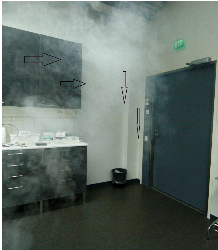
Figure 23. Direction of air flows at of existing CO 2 sensor
