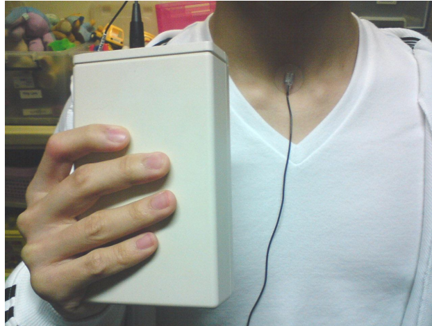
FIGURE 1. Ambulatory Phonation Monitor (APM) components: a APM unit (the white box) and a throat sensor (the small silver case glued at the neck)
