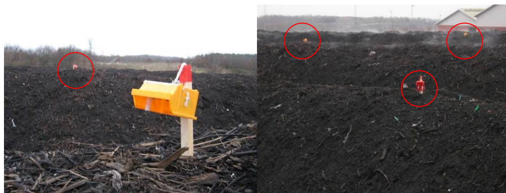
Figure 19: Placement of the passive samplers on the windrows
