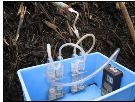
Figure 14: Detailed picture of the impinger inlet connection to the probe
