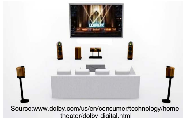
Figure 1. The speaker arrangement for Dolby 5.1-channel surround systems
