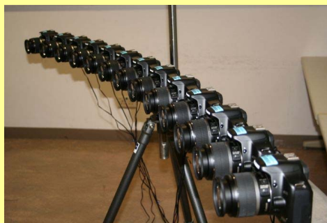
Fig. 2. Circular camera array constructed.
